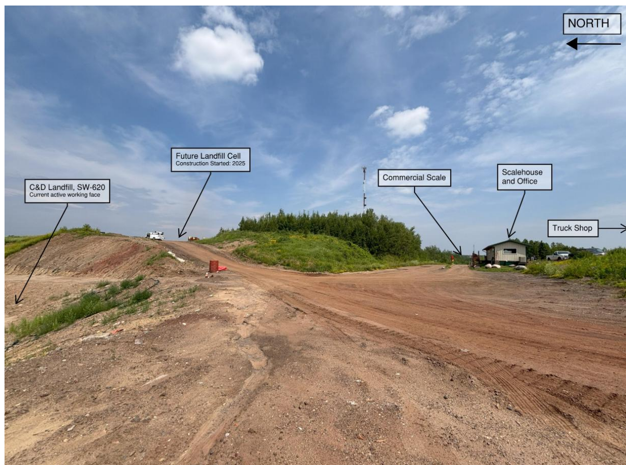
Figure 2-3: General Waste Landfill Site Layout
