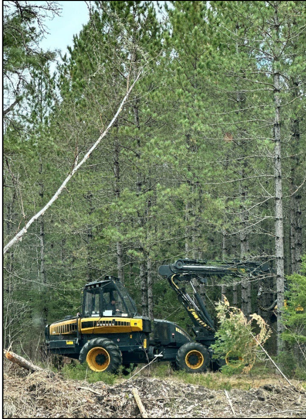
Cut-to Length Harvester processing trees on a red pine thin.
