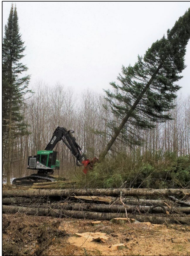
A track feller-buncher felling trees on a timber permit.
