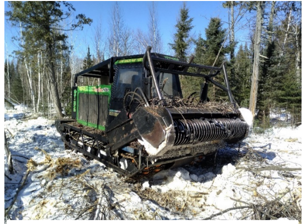
GyroTrac mulching shrubs on habitat site.
