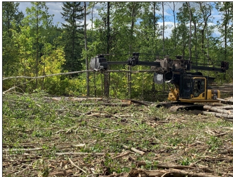
Aspen being processed with a stroke-delimber at a timber permit site.
